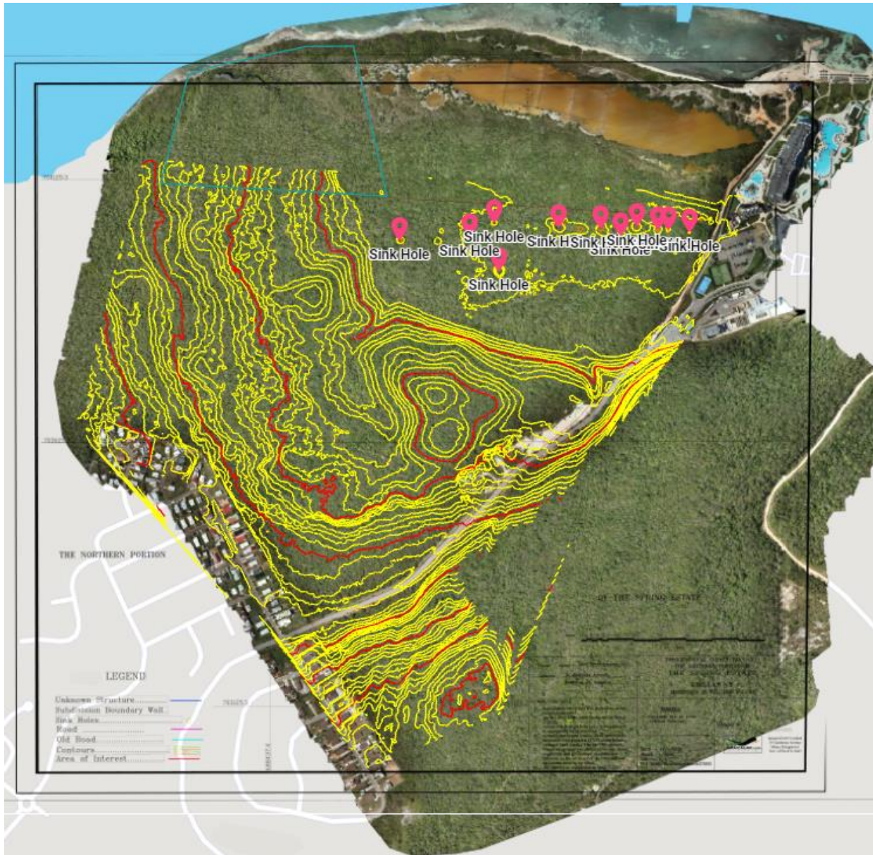
Figure 4-5: Map showing the contour lines as surveyed in the property and the mapped sinkholes in the northern boundary.
