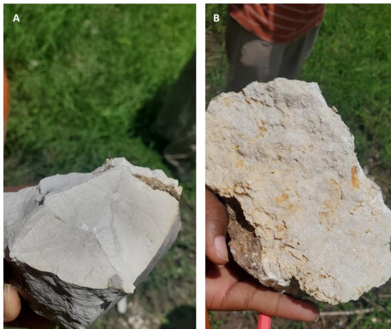
Figure 4-2: A) Limestone with dull chalky texture observed on site B) Grainstone limestone observed on site
