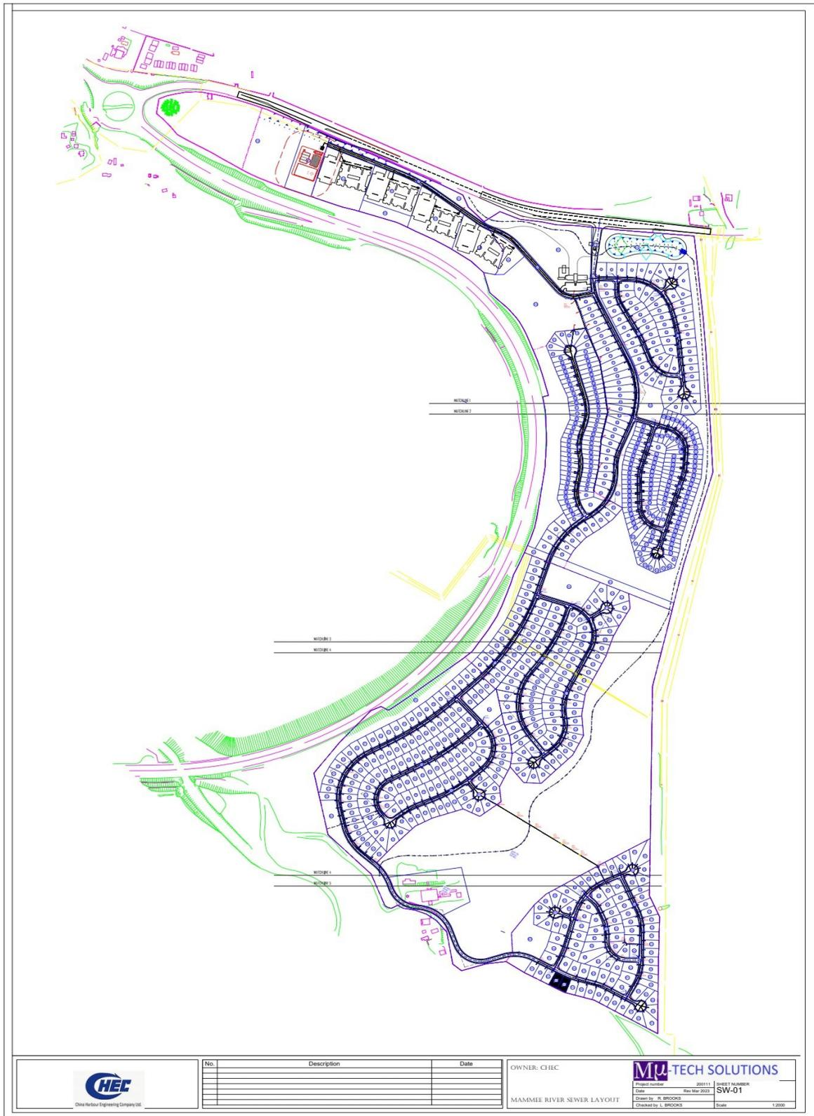
Figure 3-19: Sewage System Layout
